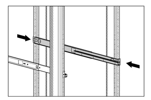
NOTE: If the UPG 1U Adjustable Toolless Rails do not snap into place, be sure that they align with the holes marked on the rack. The holes marked on the rack must be in the same location for the front and rear of the rack.
