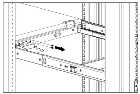
8. Attach the cable management arm to the rear of the unit with two 6-32 screws. [8 in-lbs]
