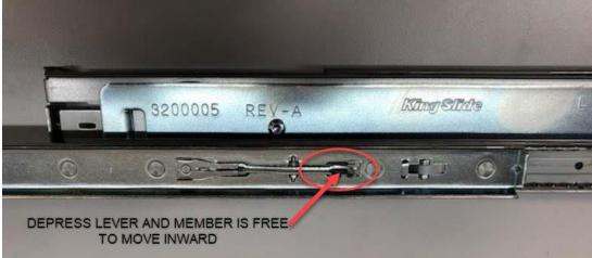
Note: Keep exposed assembly free of debris while the slide is apart! There is a light film of grease on ball bearing race, so limit touching the mechanism.
