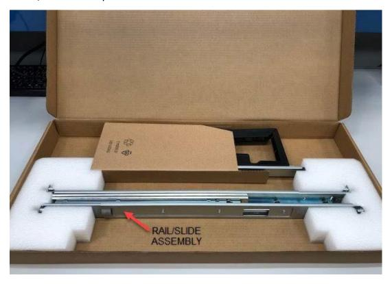
2. Place rail assembly on flat surface and fully extend slide as shown in picture below.
