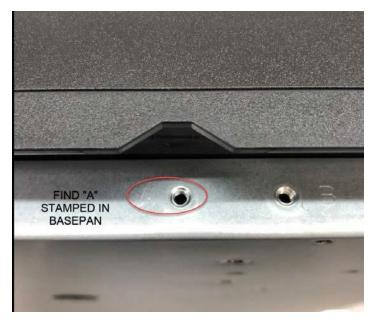
5. Place flat side of the inner rail on the side of the base pan. Align holes with pan inserts marked "A". Thread 6-32 screws (qty 2) to hold rail to base pan. Note: Use 8-in/lbs. of torque to secure screw in place.
