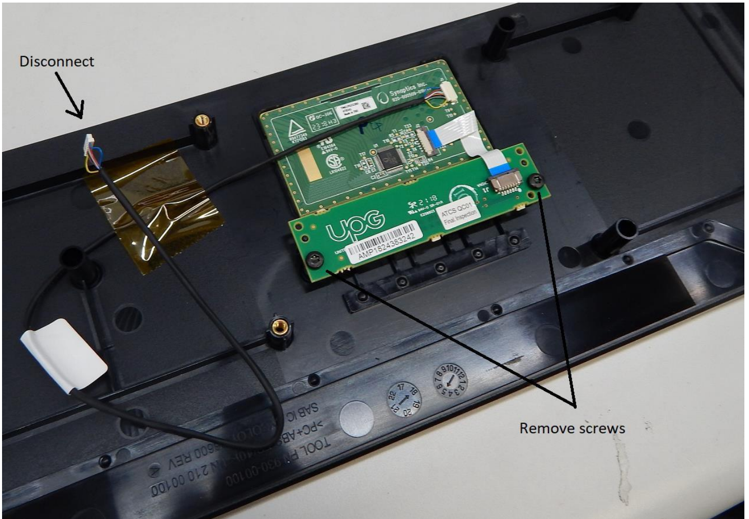
Picture 5: Touchpad Removal
