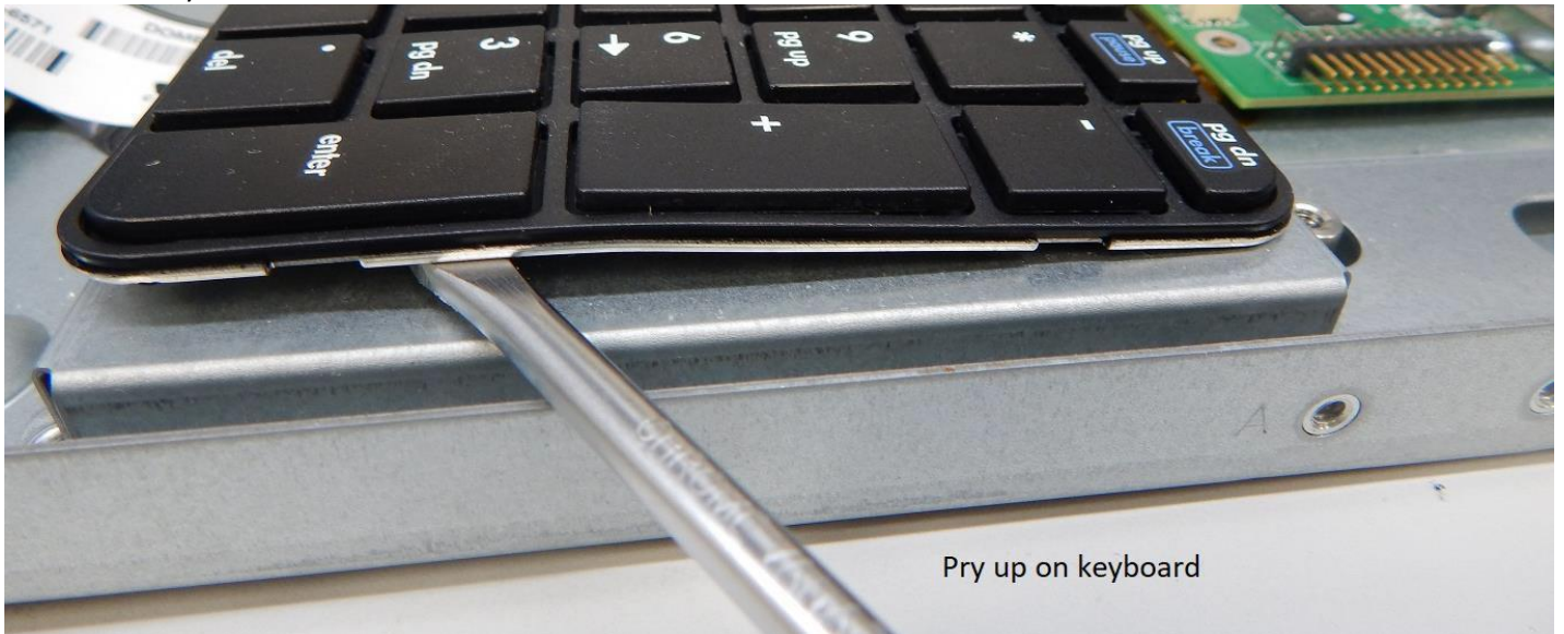
Picture 11: Keyboard Removal
