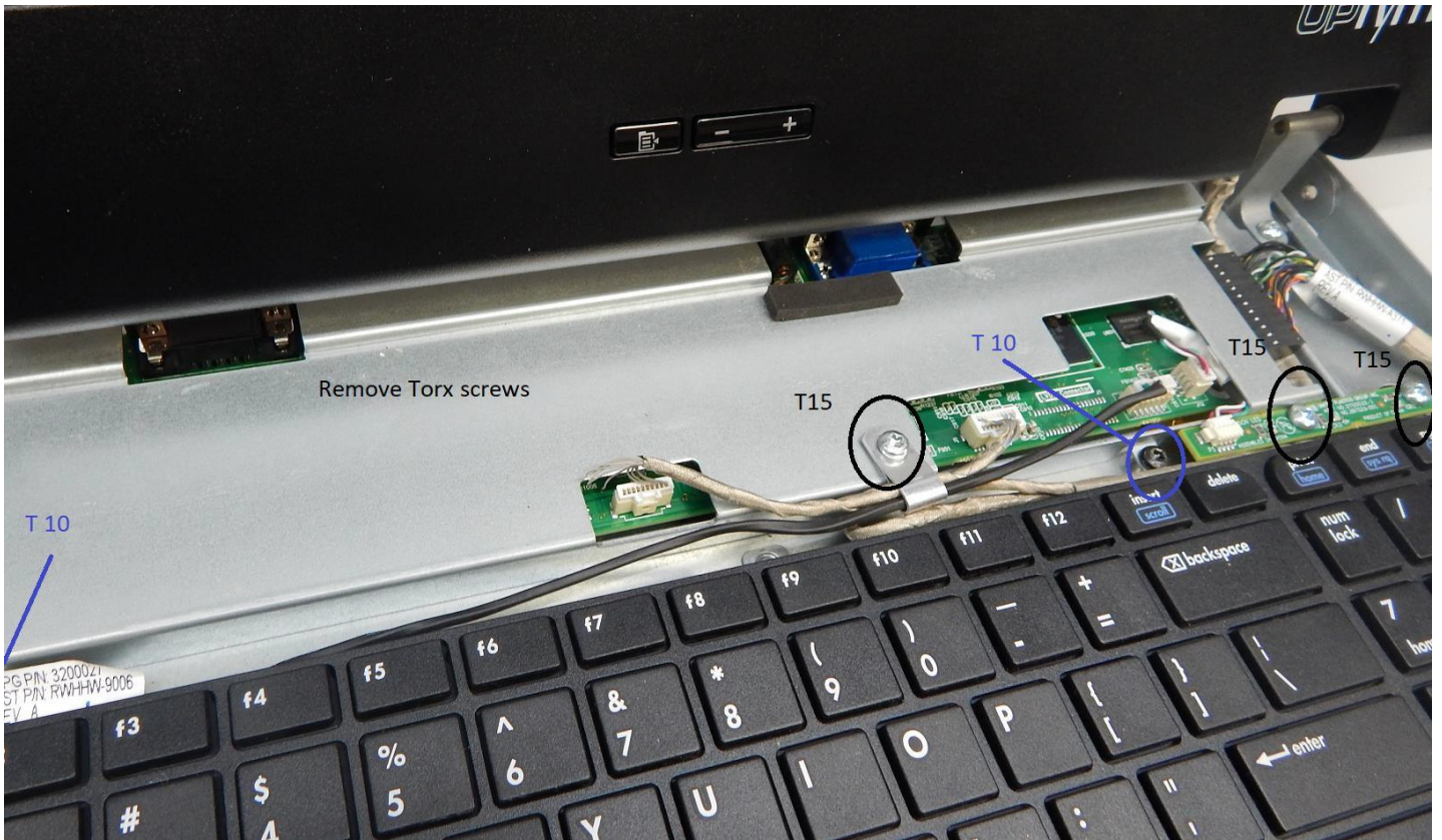
Picture 7: Clip and Cable Removal
