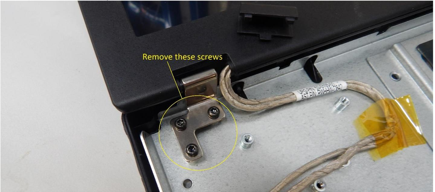
Picture 16: Display Panel Disassembly
