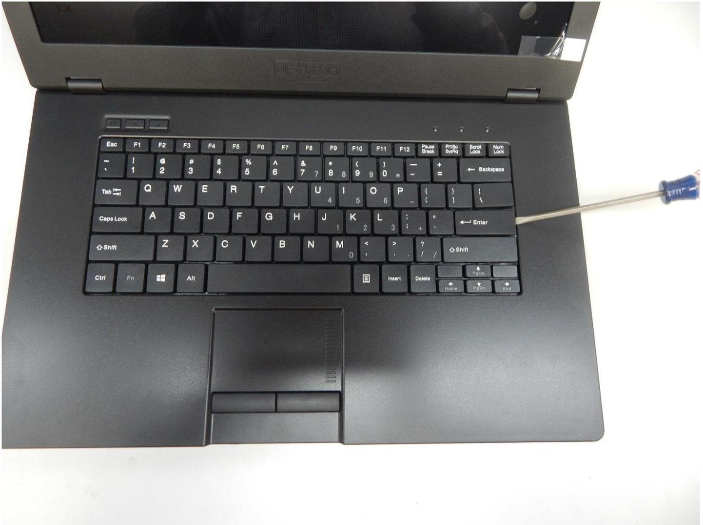
Picture 4: Palm Rest Screw Removal
