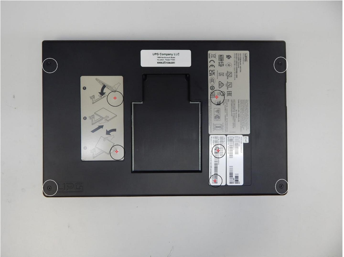
Picture 2: Bottom Screw Removal
