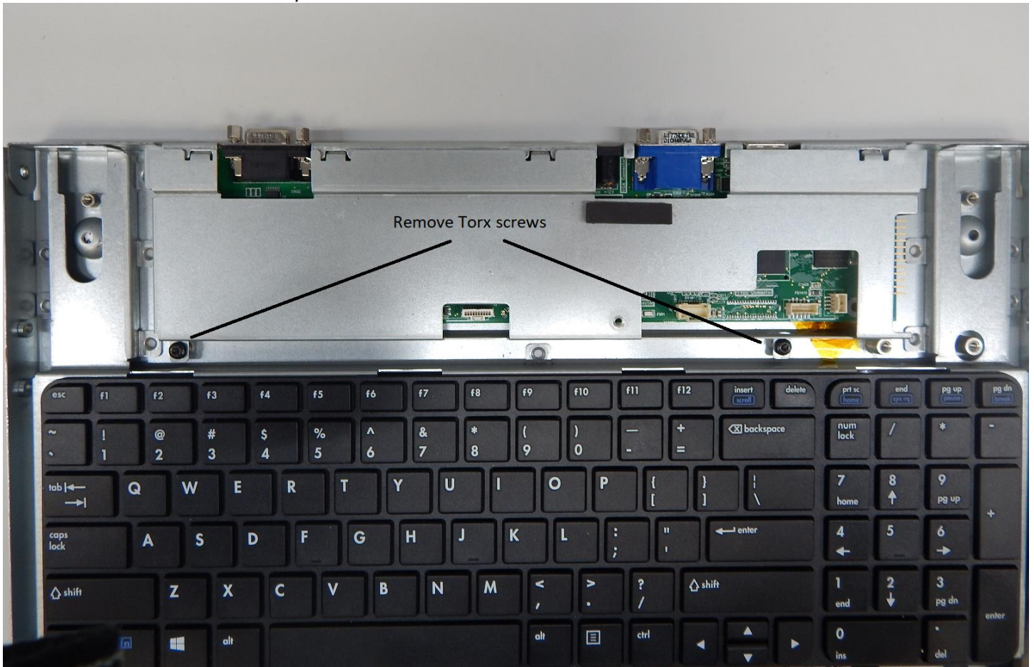
Picture 9: Metal Cover Disassembly
