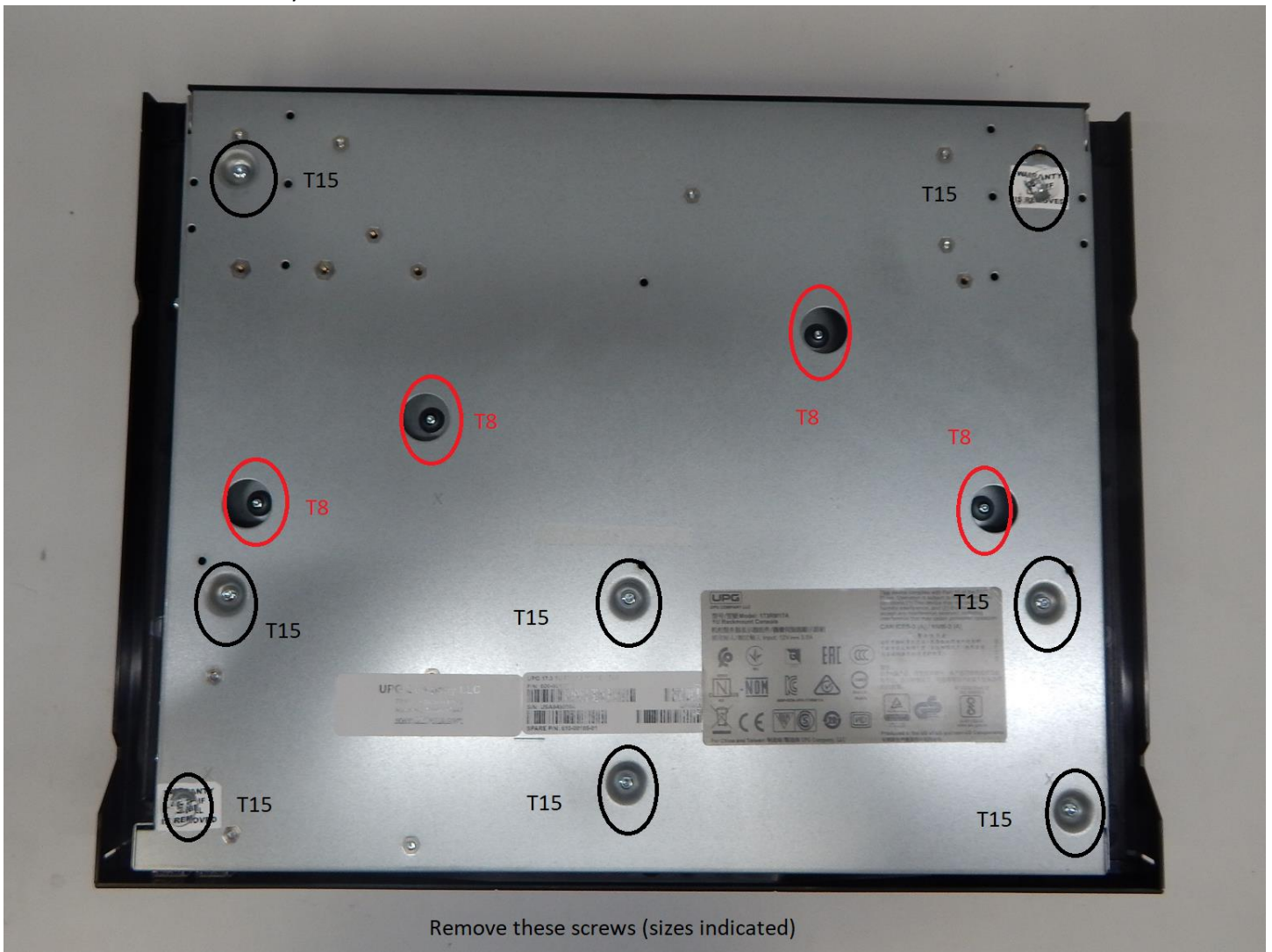
Picture 3: Palm Rest and Keyboard Screws
