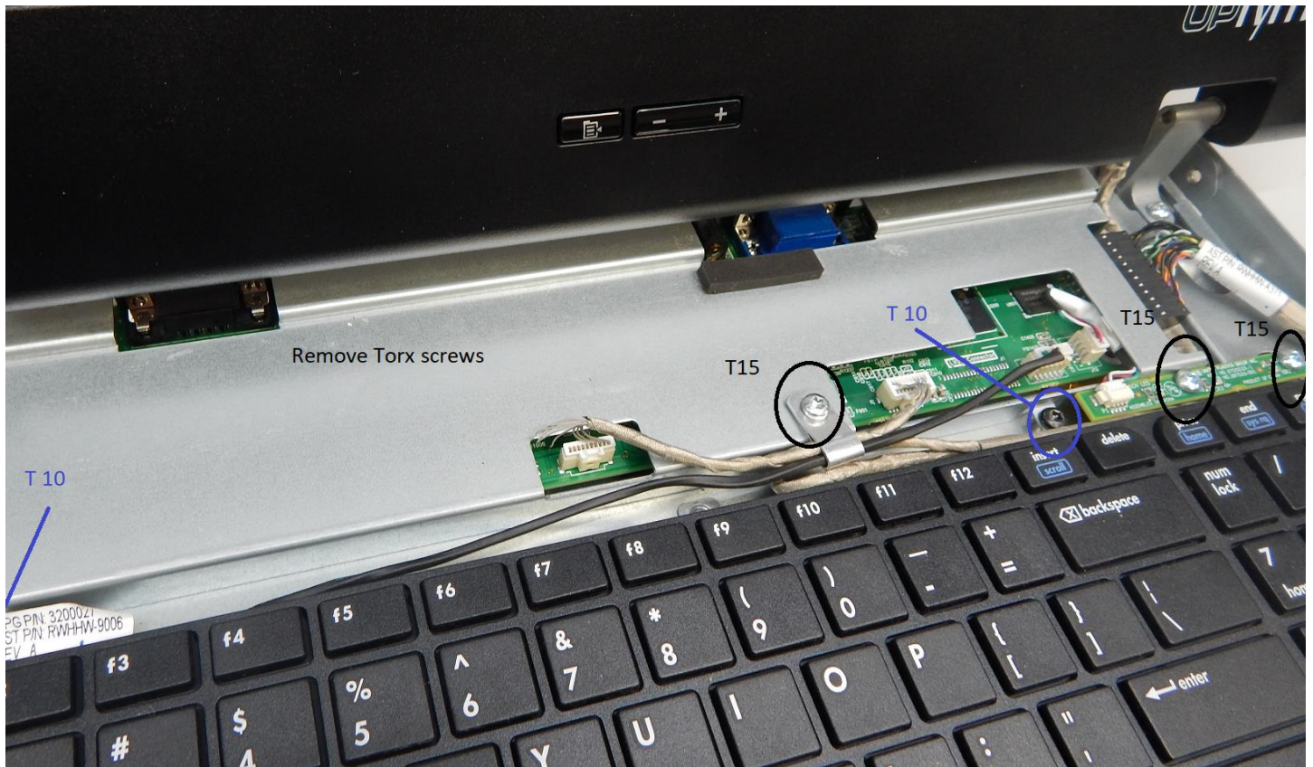
Picture 7: Clip and Cable Removal
