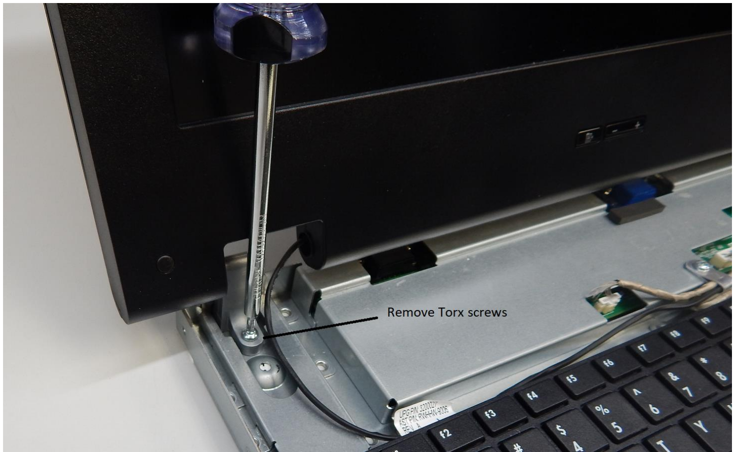
Picture 8: Clutch Screw Removal
