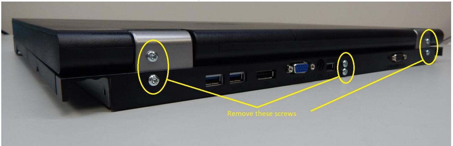
Picture 2: Console Back and Clutch Cover Disassembly
