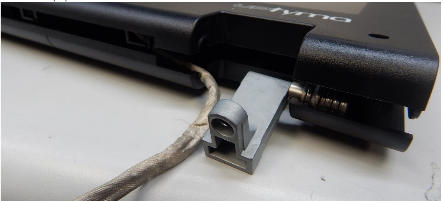
Picture 14: Display Panel Cover Removal
