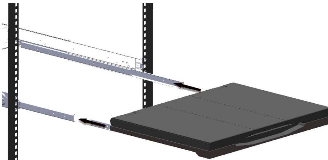
4. From the rear of the rack, slide the brace rail assembly in between the UPG 1U Adjustable Toolless Rails.
