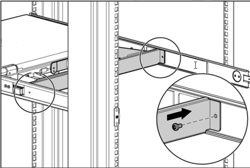
7. Remove the two 6-32 screws from the rear of the unit.
