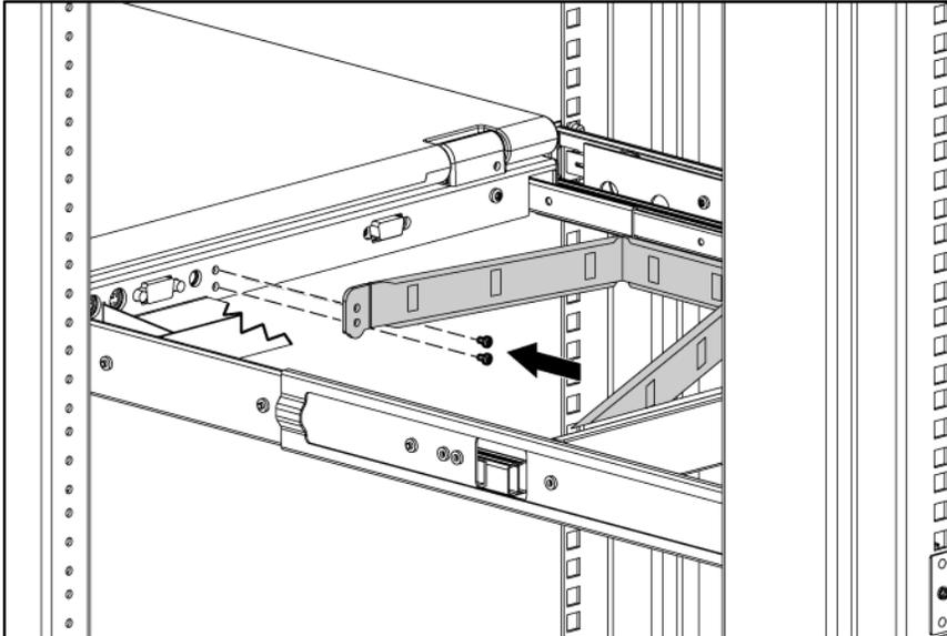
9. Connect and route the cables through the cable management arm and unit opening.
