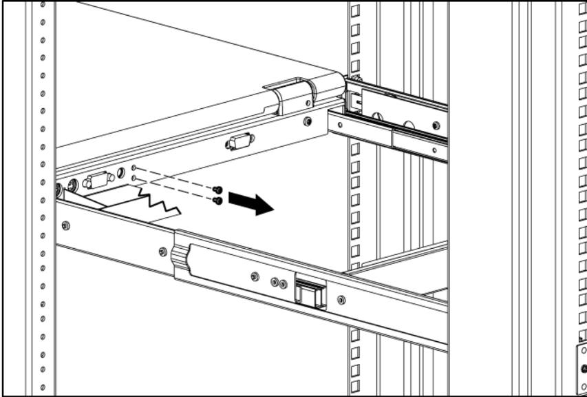
8. Attach the cable management arm to the rear of the unit with two 6-32 screws.
