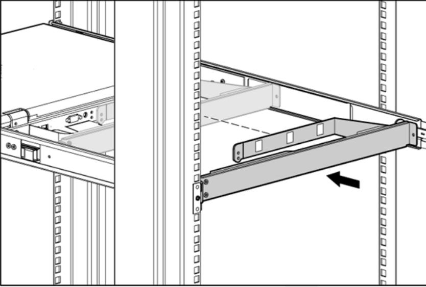
5. Align the screw holes on the brace rail with the screw holes on the UPG 1U Adjustable Toolless Rails.
